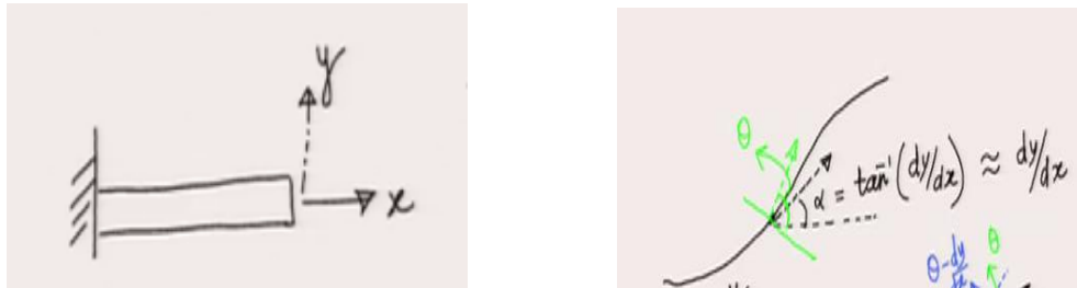
Figure 2: (a) An initially straight beam clamped at one end (b) the cross-section rotation \theta and centerline tangent rotation \alpha of the deformed beam shown
