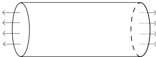
Figure 1: Normal traction applied at the ends of a cylinder to generate stretch in it.
