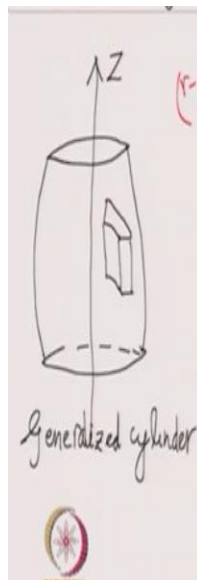
Figure 1: A generalized cylinder with its axis along the z axis. A cylindrical element is considered within the cylinder.
