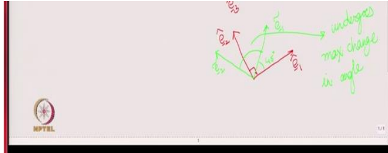
Figure 2: Line element directions corresponding to maximum shear strain ( \underline{\hat{e}}_1, \underline{\hat{e}}_2 ) shown with respect to the principal strain directions ( \underline{\hat{e}}_1, \underline{\hat{e}}_2 )
