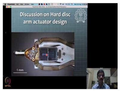
And then this is an actuator, disc actuator head, arm head here. And this head is actually the reading, there is some kind of magnetic sensors which are used to read the data on the surface of the disc. This is a magnified form of it, so this 1 mm you can see that small, very small tiny mechanism is there, and there is this flexure mechanism, compliant mechanism which is pressing the disc on the surface. This pressing the sensor not disc, the sensor on the surface of the disc.
