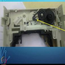
Mechanism to open and close the disc tray.
