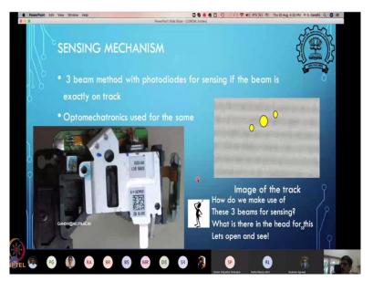
So, here when we came for the Sensing Mechanism, so first, the, again, I am explaining this, for the sake of understanding, we have these three beams that are focused on the surface of the CD, the central beam is for the data, and then these two side beams are for making sure that you are on the track, or you are in the proper data track. So how that happens is what we want to kind of see.
