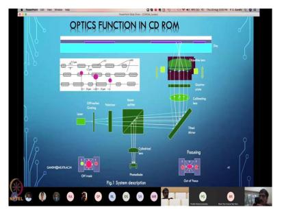
So, focusing on one side it is covering like that, and in the other, other defocus direction it will go A and C direction. So, if I consider this signal (A+C)-(B+D), then it will have a, have a error signal covered up there. And that is how I can detect whether it is in focus or it has gone out of focus. So, is that part clear? Is any question about this part again?
