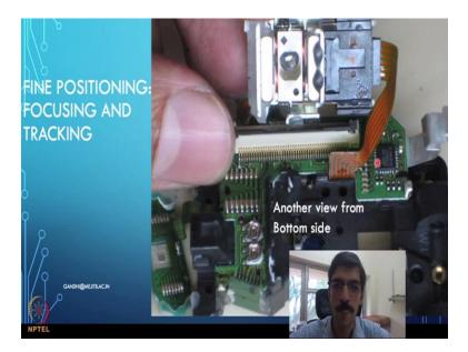
We need to have a compliant kind of a mechanism, which guides the system to go in to finer motion and why this kind of a compliant beams are needed that beams that you see here, why they are needed here. Why do not, we why do not we provided this guide by same way as we have provided with some kind of a rod or some kind of a new support to guide, the main reason for that is a friction.
