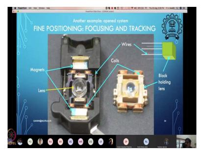
So here, you can see the all these kind of things very clearly, how the coils are placed, then there are magnets and then this is a lens from which the laser beam is coming. And then this is so the magnetic field direction one can see here. So, one can kind of like to do a lot of thinking here and saying, okay, oh, look how these coils are running.
