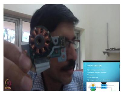
You can see this is opened up a CD servo motor and its cover you can see up here. So, this is a cover of the, of the motor and this is a motor opened. So, you can see that right this is a motor.
