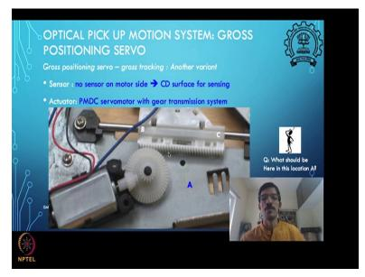
These is the other system like this as this if you see this has only two wires coming out of this motor and then there is a gear system in this like a bevel gear system and then there is this gear, think what is missing in this **location A**, **think** about that, what is missing I have removed something from there what it should have been to kind of like you can think about, so that the motion from the bevel gear is transmitted to this rack here.
