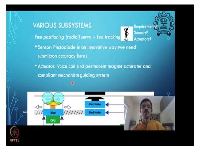
Now, let us think about the fine tracking, what are the requirements, what are the sensors, what are the actuators and we can open up and talk about that. So, the sensor that is used here is some kind of a photodetector here and actuator is some small kind of a little voice coil actuator that is sitting up here.
