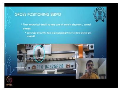
This is another kind of mechanism in which you see the same spring loaded stubs for the gross positioning system.
