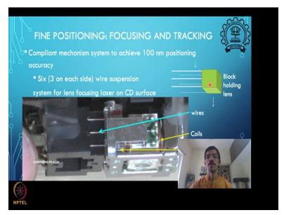
We will start looking at. So, if you see the head you will find this there is this block, which is held in the head by these wires. And you see these are the wires up here, this is a block, the block has a lens inside it. So, the lens moves up and down direction means this focusing kind of a direction, this block can move up and down, can this block get stretched front and back in this direction? Think about that.
