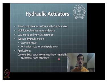
Now, we look at little bit of hydraulic actuators. So, in hydraulics you can have two possibilities; one is a linear actuators or you can have a hydraulic motor is also possible. So, we can see how hydraulic motors can be made to work actually. So, we will see that. Hydraulic actuators would be useful in the places where you need a very high force and you need very high torque in very small kind of compact environment.
