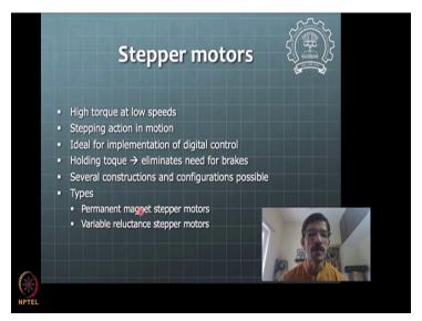
Then stepper motors are another popular actuators for mechanical mechatronic systems, we will see some of the applications soon. They are used in the places where you do not need a sensor. So, you can rely on the steps, making sure that the steps are not missed in the drive way based on the capacity.
