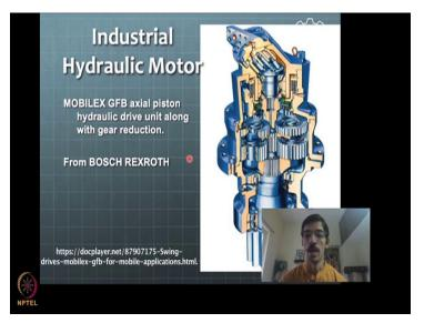
So, this is one of the open up picture of hydraulic axial piston motor. So, you can see that pistons are up here and they are operating this swash plate here, the swash plate is a rotary plate with pistons which are coming at an angle. So, you can imagine when this piston is pushed here, the torque which will be created will push the shaft it will rotate the shaft in this direction.
