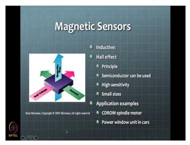
Then, there are these magnetic sensors which are based on the Hall Effect principle. The principle is very simple. You have the semiconductor which is flowing current in one direction. There is a direction of current in the semiconductor and then you have a magnetic flux which is applied in a direction perpendicular to it and then you find that because of the flow of current and in this magnetic field which is perpendicular to it, the electrons will get deflected in one direction.
