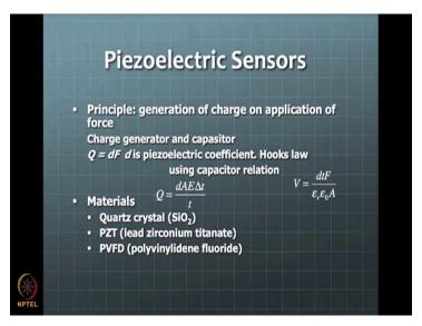
Then we can have a Piezoelectric sensors based on the piezoelectricity principle. So, this is typically the charge that is generated on the surface of a Piezoelectric element when some force is applied. So, you have two possibilities one is you can apply the force generated charge or you can have a give a charge and to generate the force both ways these piezoelectric sensors work typically.
