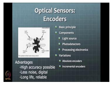
Then in the optical domain you can have is a very very what you say interesting or important sensor for a lot of mechatronics systems encoders. So, these are different from the encoder word that is used in the electronics domain. So, we need to be careful about this mechanical, this is mechanical encoders where you want the sense the position then you do this based on the principle as demonstrated in this figure.
