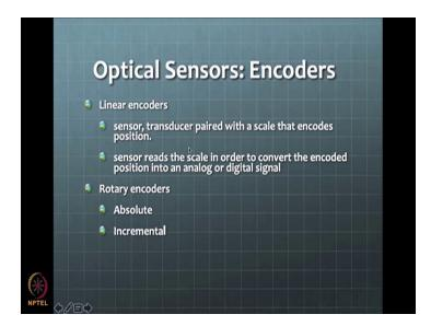
So, you can have a linear possibility for sensing or you can have a rotary possibility for sensing with the encoders. So, in the linear case, there is a scale which is having these strips on the surface. Now, as you can see, here, we are having this transmission principle and the same thing can be possible if I have a reflective principle here.
