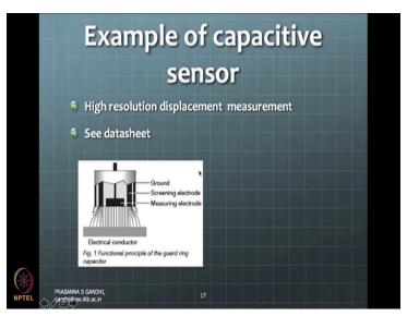
So, one of the examples of this capacitor sensor is this, this way of doing things. Where you have a surface which is electrical conductor and but it is not participating really in a capacitive measurement actively in some way. So, for example, you have this measurement electrode which is giving the field.
