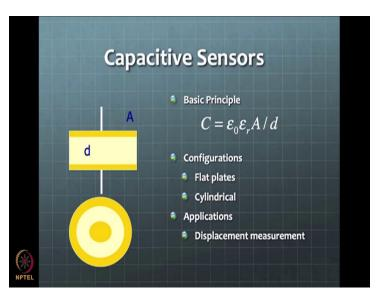
Then you can have a capacity principle to operate, the basic principle of capacitance, is  $\epsilon A/d$ . So, this A is the area of the capacitor, d is the gap between the two electrodes that are used in the capacitor. So, you can have many different kinds of configurations here, flat plate configuration, cylindrical configuration and things like that and typical application to capacitive sensors are used in are displacement.
