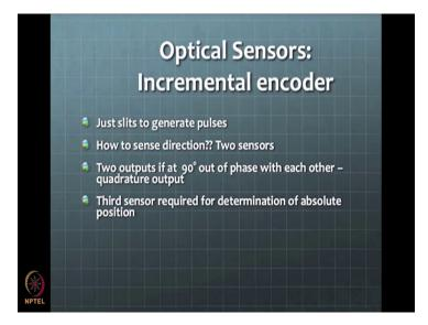
Now, we come to this question how we sense the direction of these pulses? These pulses that are coming then like know do we sense direction? So, the idea is to use instead of 1 we use 2 sensors and 2 sensors are put in such a way that outputs of them are 90 degrees out of phase with each other.
