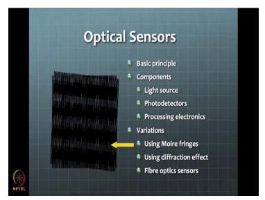
Then you can have something called Moire fringes. You might have seen you have this gate which will have to say basically, some kind of a matrix for example or gate which is having these bars which are vertical and you run other kind of a set of bars, which had slightly at an angle to it and you start moving around you can see these kinds of fringe pattern coming.
