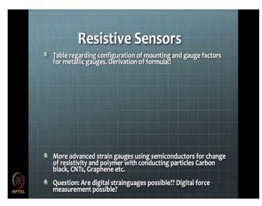
So, this table I will post in the notes. Then you can have this more advanced now semiconductor based in this silicon for example, when used as a strain sensor, the basic difference is that we are not just dependent upon the length of change there. So, suppose we
