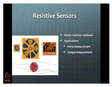
So, these are some pictures of actually strain gauge sensors for different kinds of configurations and making sure, we want to measure something torque measurement, if you want to do in place it in some, so this is called strain rosette. So, there are multiple sensors put together to get a specific measurement.
