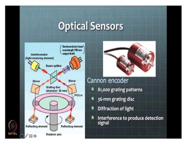
Then this is another we can have more complicated examples, where we are using some a light path with the additional light elements, reflecting elements, mirrors including that beam splitters something like that to put together very highly sophisticated sensors. So, that is possible. This is the sensors we use in long back in my PhD days we use such kind of a sensors.
