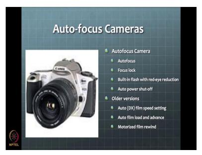
Then you can have these autofocus cameras as another mechatronics system. Now, think of this again, what could be the sensors here. So, one can see that there are systems like auto focusing. So, suppose here you have auto focusing what is, what is the sensor for the system. So, you can have the image taken by the camera on the digital screen that itself as acting as, that image itself acting as a feedback for whether it is focused or not.
