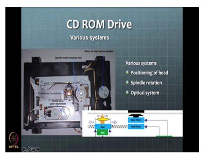
Say, for example, this is one of the CD ROM opened here. So, you can see this some of the systems here. So, we have some motors which are driving these gears here and then they are driving this slider which will slide around this around these rods here, then there will be motor on which the CD, the CD will be kept and then the motor will be rotated and then this will be sliding.
