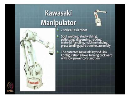
We, this is one of the techno industrial example of robot. So, many different applications can be done with these you can have spot welding application or welding application or material handling system, assembly system or some kind of actually doing some metal forming operations and things like that. So, we will not get into construction of such robots and things that, but one can see once we have some basic fundamentals of this course in terms of design strategies understood.
