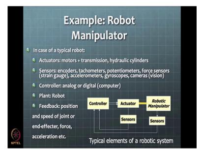
So, see first example is simply a typical robotic system if you see the actuators there are motors or there might be some a gear transmission system along with or there might be some hydraulic actuators as cylinders, hydraulic cylinders as actuators or pneumatic actuators something like that. Then you can have different kinds of sensors for a robot. Can you think of, what are the sensors?
