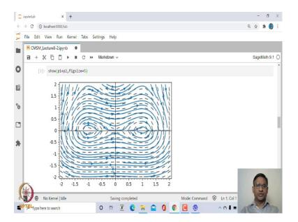
We can try to plot both these things together, the solution curve, that is, integral curves along with the slope fields. You can see here for example, if I look at this curve this is how the slope field is moving. Of course, it is quite easy to see that no two slope curves, no two integral curve will intersect.
