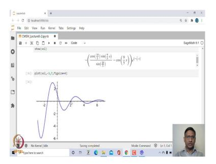
If you try to plot its solution curve, just to make sure that it satisfy the boundary conditions. You can see here, at x equal to 0, y value is 1 and x equal to 2, y value is 0. So, this is the solution curve.
