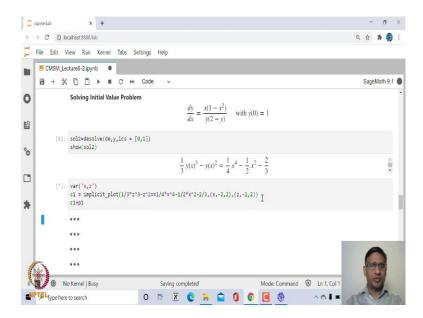
So, if you have to solve this, all you need to do is, again you call desolve and you need to mention the initial conditions. You can even say ics is equal to initial condition is equal to 0 comma 1. So, this is x0, y0, that is, how the initial condition is given. So, let us ask it to solve. This is what you get, this is the solution.
