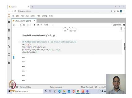
So, first thing we will look at how to plot slope fields associated to this differential equation. When we say slope field, what does it mean? dy by dx is nothing, but slope of the curve y equal to f(x). So, this is your y equal to f(x)
