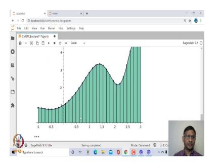
So, what you have to do? When you are dividing into 30 equal parts, you take first two parts and in that you fit a quadratic interpolating polynomial, take the next part, fit the inter, quadratic interpolating polynomial, and so on.
