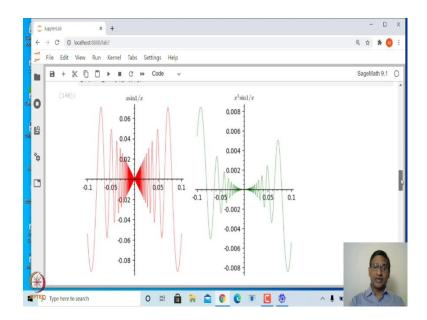
This is a graph of  $x \sin(1/x)$  and this is graph of  $x^2 \sin(1/x)$ . So, in this case if you look at this is somewhat very sharp turn here sharp edge here in corner I should say. In fact, you can draw a line y = |x| and you will see that this near 0 the value is very close to that mod x function which is not differentiable at x equal to 0.
