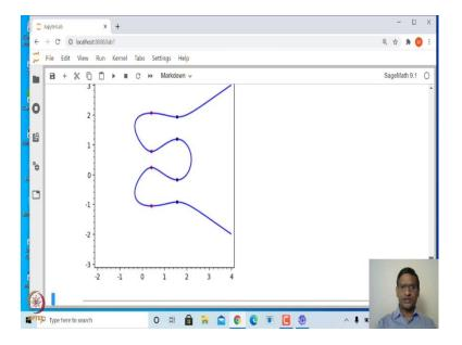
These points you will see here these are the 8 points at which the tangent is parallel to x axis. Of course, you could have also plotted the graph of this the tangent at these points fine.
