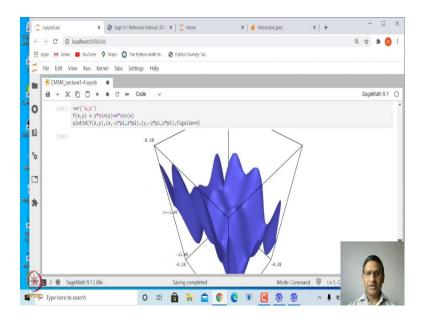
Now, when you plot the graph of this function, this is the surface. Now, how does one build this surface? So, if you actually take the slice of this surface by z planes various z planes or planes parallel to x-y, then you will get curves. This curves you project it on x-y plane they are called contours.
