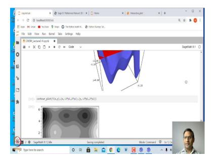
So, let us plot these contours. So, Sage has inbuilt function called  $contour\_plot()$ . And again you supply the same option like control plot of f(x, y) and x going from -2pi to 2pi, y also varying from -2pi to 2pi.
