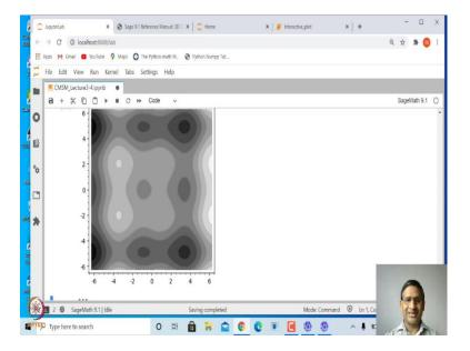
So, when we do that, it will plot default some contours. But this has actually shading inside. The shading depends upon the height of the contours, so that is why we can say graded shading.
