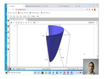
So, that is what you can see here. So, it has been rotated by an angle pi that is what you see here half of the paraboloid. And, this is the parametric equation of the surface in terms of u and phi. The phi is the angle of rotation right. So, that is very nice, whatever by angle by which you want to rotate you can do.
