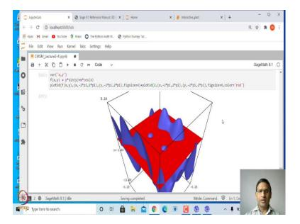
So, color equal to let us say red inside single quote right. Now, you can see here, this is the intersection of this plane by z=2 plane and the intersections are going to be curves. So, this when we project these intersections which are curves which we project on x-y plane, this curve is called contours right.
