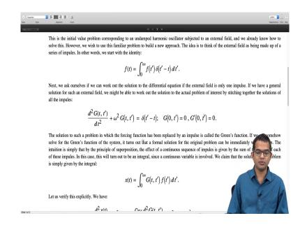
So, now we exploit the principle of superposition. Suppose we work out the solution not for this original differential equation as it is, but for this differential equation where we have only a delta of t prime minus t sitting on the right hand side. So, instead of having the full function f of t which is a hard problem in general so instead of that we will just put in a delta function there.
