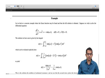
Let us see what happens when you have a you know an undamped harmonic oscillator, and when you put your external forcing function is sin omega t x of 0 equal to 0 x prime of 0 equal to 0. So, it is exactly like the previous problem. Now, I have provided what this f of t is. If I take it to be sin omega t, then the solution is given by this integral.
