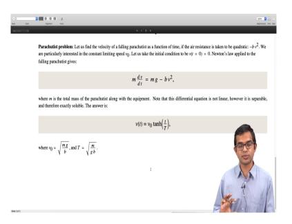
And the answer here turns out to be, so let us very quickly look at this. So, we have m dv by dt is equal to mg minus, so we have m dv by dt is equal to mg minus bv squared. So, let us divide throughout by b. So, we have m by b, dv by dt is equal to mg by b minus v squared. So, we have defined mg by b, mg by b as v naught. So, we have the equation and m by b is g T square.
