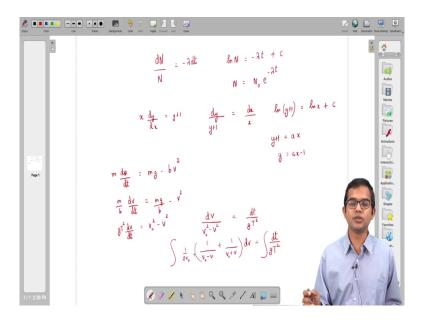
So, we can write this as d N by N, d N by N is equal to minus lambda dt is equal to minus lambda dt. So, integrate both sides, so you get log N is equal to minus lambda t plus some constant. So, therefore, N is equal to you can absorb this constant into this and it is just N naught times e to the power minus lambda t, right. So, a very familiar differential equation. I think most of us must have seen this, ok.
