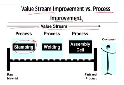
Now what is it? That value stream is actually a series of processes where just we discussed that there are 3 processes stumping, welding, and assembly. So start with stumping, that is taking only one second, then welding is there and then finally 2 cells are there where you are doing the assembly operation. So these are the various processes and total of those processes is known as your value stream.
