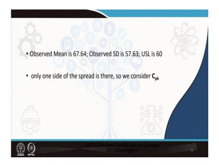
Observed mean is so, when we calculate you will see observed mean is 67.64, observed standard deviation is 57.63, USL is 60 ok. Only one side of the spread is there. So, we consider C pk ok. Now, you have to be very careful with this data because here the time gap is just 5 minutes. So, you will question every data point.
