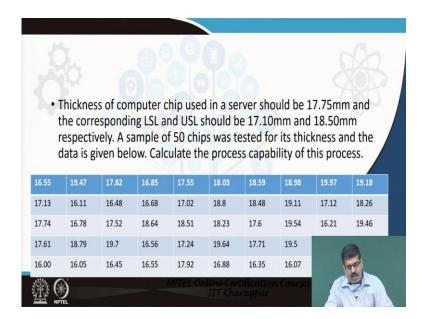
But, I think I have this is another one, thickness of computer chip used in server. This I am leaving this problem also with you, a sample of 50 chips was tested for its thickness and the data is given below, calculate the process capability of this process.
