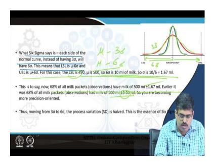
What Six Sigma says is each side of the normal curve, instead of having 3 standard deviation will have 6 standard deviation. That means, that the lower specification limit that is between mean and this value, that is between the mean and the LSL mid mean and the USL is now not mu minus 3 sigma. It is now mu minus 6 standard deviation; ok.
