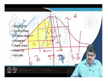
What is Six Sigma? Ok; 68 percent within 1 standard deviation, 95 something within 2 standard deviation and 99 within 99.996 within something within 3 standard deviation on both sides; on both sides, one is on both sides, ok. What now we are saying? We are saying this side is not 3 sigma, this side is 6 sigma.
