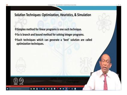
Simplex method for linear solving linear programming type of problem is one such technique which generates optimal solutions. So is branch and bound method for solving integer solution, integer programming problems. And these techniques they generate the best solution on a given constraint and they are basically these techniques are known as optimization techniques. Some problems in real life are very complex.
