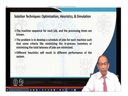
The machine sequence for each job and the processing times for those jobs in the respective machines are already known. The problem is basically to develop a schedule for those jobs for each machine such that some criteria like say minimizing the in process inventory or minimizing the total lateness of jobs is met. Different heuristics will result in different performance of the system. And depending on what the managers want the rules of thumb will be deployed.
