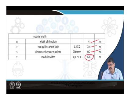
Now, having said that let us go to module width we have run we have done this formula of module width was what. Module width formula was this one aisle plus clearance plus 2 pallet width; ok. So, let us go to module width calculation. Width 2 pallets aisle that is clearance between pallets. So, module width is 6.6.
