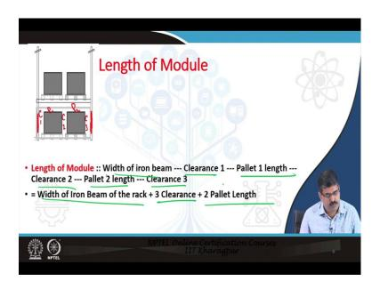
What is the length? Length of the module is like this length of the module is the width of the iron beam. Remember the first diagram that we drew width of the iron beam the width of this iron beam clearance here.
