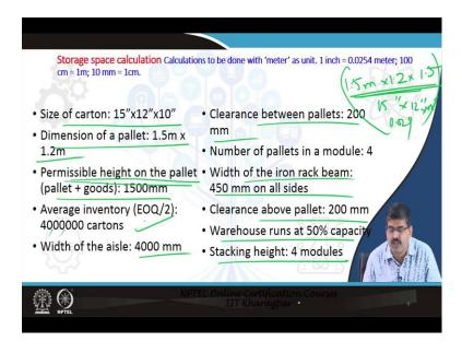
This is I would say, this is self-explanatory but you can definitely pause, read, go through again; pause and check-up, it is self-explanatory problem but we will go through it; ok. Storage space calculation calculations to be done with meter per unit as 1 inch is equal to 0.0254 meters or the 100 centimeter 1 meter 10 millimeter 1 centimeter given it for easy calculation.
