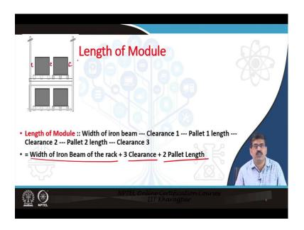
3 clearance, 2 pallets; what was clearance? Clearance 1, clearance 2, clearance 3 ok. So, same thing here yeah. Module length width of iron beam, length of pallet that is 2 pallets and 3 clearances. So, module length is 4.05. So, module area is this um. So, module width module area is module length into width 26.73.
