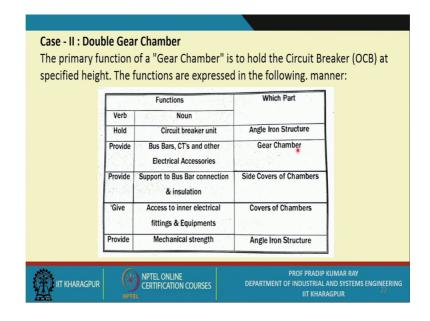
As far as the double gear chamber is concerned; the primary function of a gear chamber is to hold the circuit breaker. You have the you need to identify the primary function, then you move to the secondary function, and then if required you identify the tertiary function.
