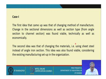
Then so, this is the first idea; that means, we have to change the method of manufacture and the second idea was that of changing the materials.
