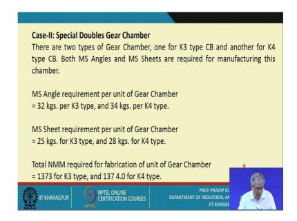
So, this is your materials requirement, and with referred with reference to the special double gear chamber we have the 2 types of gear chamber. One for K3 type you know circuit breaker, and another for K4 type circuit breaker. Both MS angles and MS sheets are required for manufacturing this chamber.
