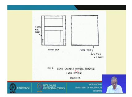
And this is the new design for the gear chambers.
