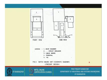
So, this is the schematic diagram of the structure. So, this is the front view, and this is your side view. So, you have the gear chamber, this is the gear chamber, these are the circuit breakers, these are the circuit breakers. These number 3 is the cable boxes, and number 4 is your pedestal, and the 5 is essentially the time. So, this is a schematic of the presentation of the entire the fabricated body, and as per as gear chamber is concerned this the drawing you have with covers removed.
