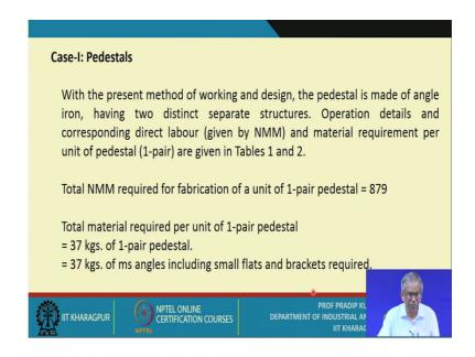
Now, when we refer to the pedestals, with the present method of working and design. The pedestal is made of angle around having 2 distinct separate structures. If you refer to the drawing you will get this details. Operation details and the corresponding direct labour given in normal man minute. And material requirements per unit of pedestal are given in tables 1 and 2.
