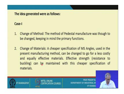
So, all this questions are there. So, the idea generated where as follows change of method that is the one idea; that means; you need to change the method and the change of materials. So, the cheaper specification of MS angles used in the present manufacturing method, can be change to go for a less costly and equally effective materials, is it?
