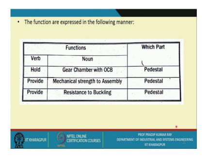
So now, if you put it in a verb and noun form to avoid ambiguity the function would be written as hold switch boards. So, now the functions are described in terms of the verb and noun. So, the verb means hold provide, provide. And the noun is you know the hold gear chamber with circuit breakers, provide mechanical strength to assembly, provide resistance to buckling.
