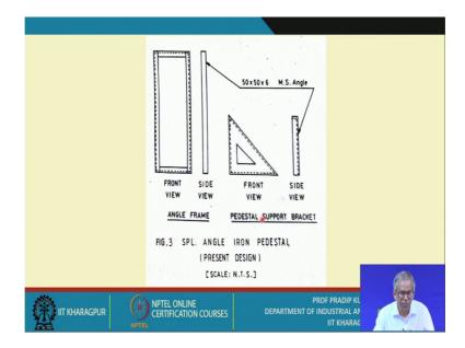
And then this is the special angle iron pedestal, when you refer to the present designed. So, first you refer to the present design, get the details. So, this is the front view, this is the side view, this is the angle frame. And for the pedestal support bracket, you have these the front view and this is the side view. And this is the mile steel angle that is 50 by 50 into 6. So, all these detail informations you have.
