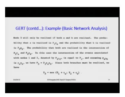
So, node 3 will be will only be realized if both a and b are realized. The probability that that a is realized is capital as I already said; so, considering the simplest case of P 1 and P 2 being equal we are that is the simple one.
