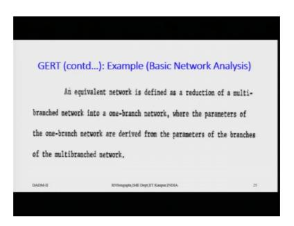
Now, we will basically have to convert them into the equivalent networks. So, an equivalent network would be defined as a reduction of the multi-branched network which we already have into the basic AND, OR, exclusive-OR, INCLUSIVE-OR nodes and network such that the complexity of the diagram is reduced, yet it basically has the same logical sequence of the output and the input combined together in the same way as it was earlier; earlier means before you reduced.
