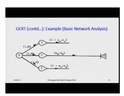
So, we have from the source 1, 2, 3 outputs the probabilities are one for the second one the cumulative the equivalent probabilities p E, equivalent time is t E and the corresponding probabilities and time periods for the so called paths emanating from 1 and 3 are corresponding to 1 minus p a and 1 minus p b because you have that one part is realized another part is not realized would be given by 1 minus p a and similarly for the third part it would be 1 minus p b.
