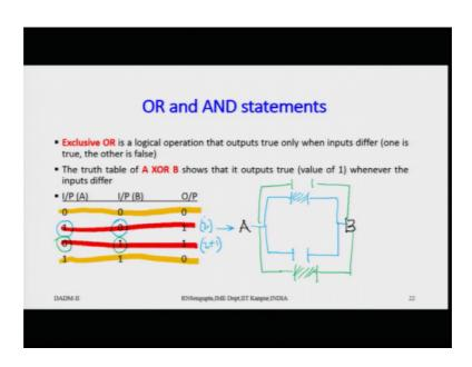
Now, I will consider very simplistically the AND, OR statements and AND, OR logical statements because based on that we will try to basically build up the model. So, the concept of Exclusive OR is a logical operations or process that outputs true only when inputs differ. So, when the inputs are like this.
