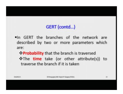
In GERT, the branches of the network are described by two or more parameters which are what is the probability that the branch will be traversed. So, obviously as I said product being successful 40 percent, product not means that successful 30 percent and product be in a failure by can be 20 percent.
