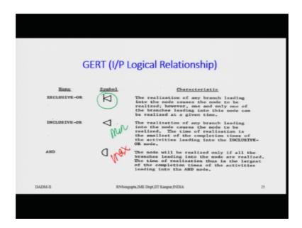
Now, in this case we will formulate with the symbols for the GERT. So, the Exclusive-OR would be a triangle operator with a vertical line. So, the realization of any branch leading into the node causes the node to be realized. However, one and only one of the branches leading to this node can be realized at any given point of time. So, it is an Exclusive-OR.
