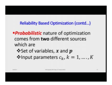
The probabilistic nature of the optimization comes from two values which I have already mentioned, it is from x which is the decision variables and the p is the parameters which are external to the system point 1. And it also comes from the input parameters which is c k which is the set of the right hand side inequality which you have for the list of non-deterministic constraints which are already there which is c k, k is equal to 1 to capital K.
