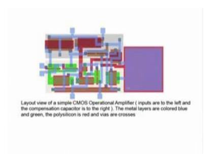
Now, if I ask that, let us see this is a CMOS operational amplifier layout; that is a layout of CMOS operational amplifier. How metal layers are colored blue and green; the polysilicon is red and vias are as crosses. That is the layout of CMOS amplifier.
