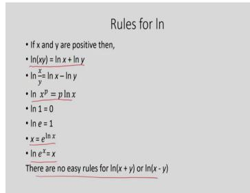
Now, here are certain rules for natural log or ln. If x and y are positive, then  $ln(xy) = lnx + lny; ln(\frac{x}{y}) = lnx - lny; ln x^{p} = p lnx; ln 1 = 0; ln e = 1; and x = e^{lnx}$ , that we have just seen; and  $ln e^{x} = x$ .
