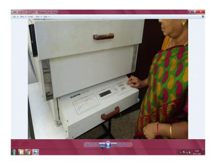
So, one lady is operating one I do not know what exactly it is. It looks like it is some UV curing equipment for this printed wiring board where there is some heating and. The thing important thing to notice here is you have a profile for ramping up the temperature and ramping down the temperature. At this point you probably do not actually require a very complicated LCD display. All you need to do is you just need to you know make these points and probably there is a small bit of selection.
