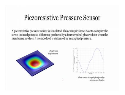
This is the first example that we will talk about. This is an example of a diaphragm that you can see over here and we apply a particular force on the top from here and we have a piezoelectric sorry piezoresistive material in this case over here with different types of doping.
