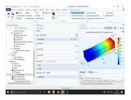
So, let me just go to compute. So, now, we can see that the displacement which is in order of nanometers. So, what you see right now is an exaggerated view of what is happening within it.
