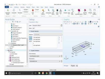
Then, we have electrostatic again we use the material model piezoelectric material model and we give the electric potential in the bottom. So, you can see over here in the bottom part I have given the piezoelectric material property and then in the top part I have given
