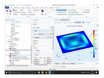
So, now you can see the stresses that is being developed on the surface and along with the deformation. So, says you how the deformation is going to be and this is a skilled version of deformation. So, if you want to see the actual deformation, make the Scale factor as 1. The deformation that the this stresses that you can see you can also change
