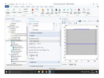
So, it actually shows the equation. For example, in linear structure linear elastic material it shows you what kind of equations you are going to solve for. This is the most important part of COMSOL that it is a very open software. It does not hide you what is it solving for.
