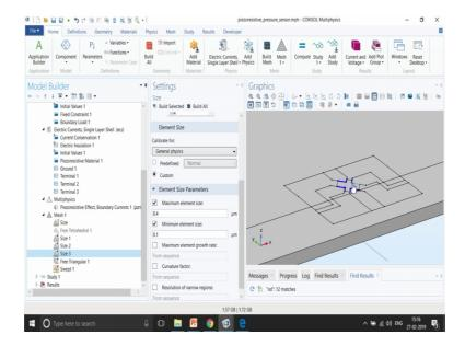
And, then finally the mesh part this mesh part is always interesting because there are many different ways or approaches to mesh this particular domain. The way it has been model over here is they have given different different meshing elements to each of the domains. So, you can see the piezoresistive material is having maximum elements size is 2 micro meters.
