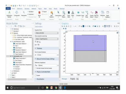
So, here it is important to know that we have not selected the aluminum part within the electrostatics. So, this is the aluminum part, but we have not selected over here because we know that the potential within this aluminum domain would be same. They would the electric field within this aluminum domain is going to be 0.
