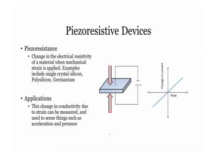
So, let us go ahead with the piezoresistive device. This is a very interesting type of a device because over here based upon the forces that we apply or this stresses that are
