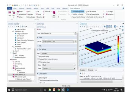
The first thing is the electric potential. So, we give a high potential in the bottom and ground it in the top right. So, you can see a nice deep or deep in through the from the bottom to the top, a linear deep.
