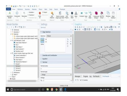
So, in the next part is from where the potential has been given. So, you can see in the terminal 1 a particular voltage of 3 volts have been applied over here. So, I am zooming a part of piezoresistive materials only. So, terminal boundary condition have been given over here and a ground has been given on the opposite side. So, the current is going to flow like this to this domain to the piezoresistor and then finally, it will arrive over here.
