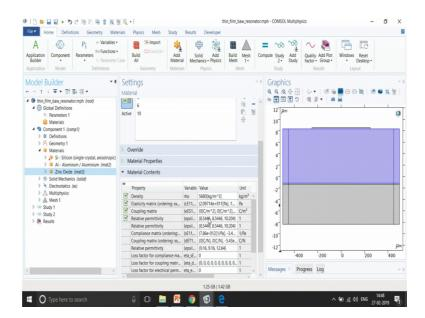
This is again elasticity matrix coupling matrix is a tensor and again the relative permittivity is n anisotropic which is more in z-direction as compared to x and y.
