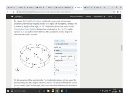
So, if you want to give a particular angle to the poling directions you can actually use a rotated systems right with the different different angles that you can see over here different material properties.
