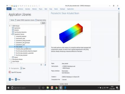
So, I just go to COMSOL, I go to File, Application Library and over here I search for shear bender. So, this is example model this is again a very example a very nice example model because it talks about the poling direction being different as what is given from the by default.
