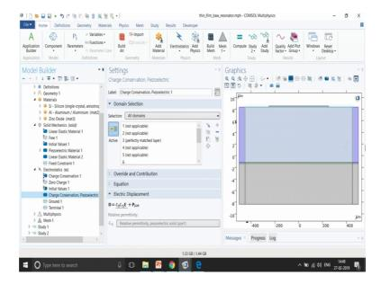
And, we are again giving a piezoelectric material model for the top part we are giving a terminal boundary condition.
