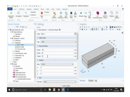
So, let me go from top to bottom. So, in the component section first thing is to make the geometry. So, I just go ahead make the blogs and make the geometry, I first make a block and they are introduced the centre domain using layers over here.
