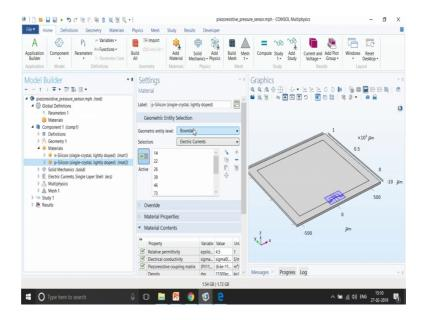
Again, for the p-type; now, the interesting part comes in to picture that we are using boundary. So, we have done away with the modelling volumetric approaches, but now we are going to model the p-type silicon as boundary.
