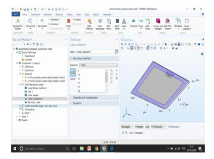
And, then the next part is the physics. So, in this case you can see that solid mechanics domain has been assigned. In the case of shell only a shell would be assigned. We give a fix constants on the bottom part; this is a bottom red part that you can see over here. So, in the boundaries we give fix constant and give a boundary load on the top part.
