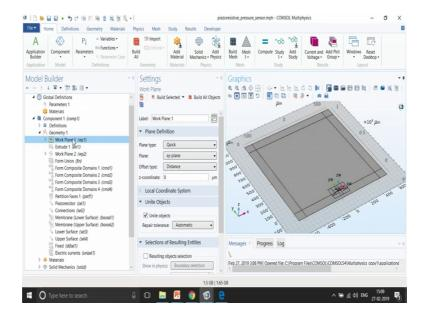
So, first thing is to make work plane and then if as you can see over here in the workplace we created a small-small geometries.
