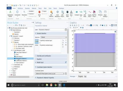
The physics setup is should be simple. So, we are using for zinc oxide you can see over here. We are using a piezoelectric material property over here and then you are using stress charge form and, in addition to it there are some kind of losses.
