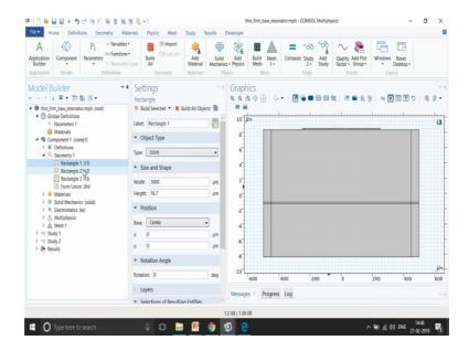
So, first thing is to make the geometry. So, I use rectangular 1, rectangle 2, rectangle 3 to make the geometry. The next part is the materials. The most important part is the materials.
