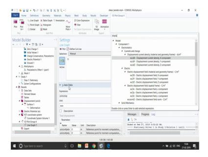
So, if I want to search I can also search over here. So, I go over here and the search for displacement and there are many other variables. So, right now I am looking for total displacement right. So, I just use the total displacement over here.
