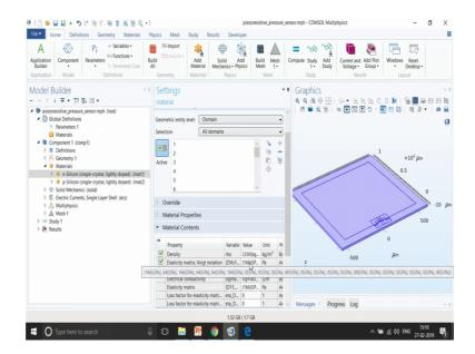
And, then we extrude this particular structure from top to bottom and then we do one more work plane I think this to extrude some ok. This is to extrude in the other direction. So once you are done with a geometry the most important part is to assign the materials.
