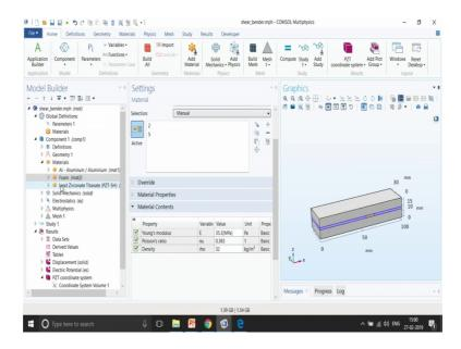
Then, we have foam which is on the left and right that you can see in the blue part in the screen and this again is a scalar material properties where you can see.
