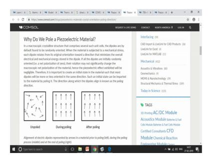
And, once you give a particular external electrical field you will see the dipoles to be arranged in a particular direction quite. So, during the poling it so, it is a particular direction that is along the electrical field.
