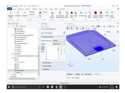
Andm, then the free triangular top boundary has been model. So, not the complete volume, but only the top boundary has been modeled over here.
