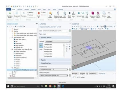
So, next part is again the multi physics part that couples the structural mechanics with the electro electric currents interface.
