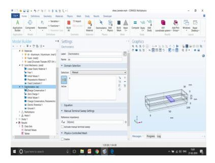
Next part is a solid mechanics part and over here again we use piezoelectric material over here the way that we define earlier we give this works as a actuator beam that is why we give a fix constant on the left side ok. So, it is going to act as a beam. So, if there is going to be some deformation it is going to deform in the up or the bottom.
