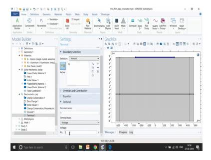
So, we use only boundary condition on the edges of your aluminium plates. So, here you can see in the bottom plate, we have given at terminal boundary condition with a voltage of 1 volt.
