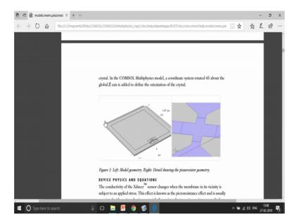
So, this is the actual structure that you can see over here. This is a diaphragm over here and then we have the piezoresistive structure over here which is kind of a Wheatstone bridge kind of a system, where we give a particular voltage on the one side and ground
