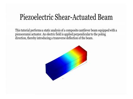
So, let us go ahead with one more example of piezoelectric shear actuated beam. So, these in this example what we are going to do is, we are going to have one piezoelectric device in the middle, which is covered with foam on the left and right side and then we have two structures elastic structure elastic models on the top and bottom and we are
