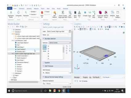
The next part the most important part is now how do we handle the electric currents in a boundary? So, again you will see that we are done away with the volumetric approach.
