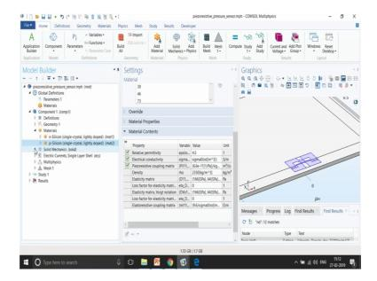
So nd is actually the density of the material, that is what understand. So, once you understand how the materials have been defined, so, over here also you have coupling matrix which is a 6 by 6 tensor.
