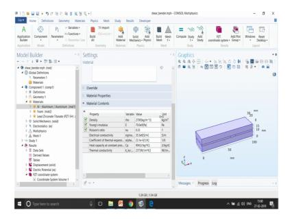
And, then I assign the material properties most important, aluminum domain in the top and bottom. You can see the blue part the top and bottom is aluminum domain and here you assign it as a scalar material properties ok.
