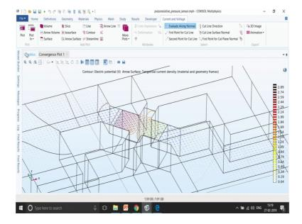
So, you can see that the voltage that I have applied is over here somewhere over here and the colour represents the per volt sorry the colour of these counter plots represent the voltage that you can see over here. And, the arrow plot actually represents the flow of the current from the voltage part over here to the ground over here. So, this is the flow of current that you can see right.
