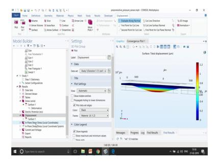
This plot talks about the displacement. This makes sense because it is having bounded surfaces on the edges. So, all the forces are going to accumulate in the center as you are going to pull it down on the center.
