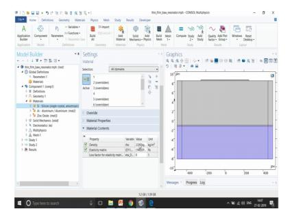
So, let us go to silicon that is the bottom part; and you can see the density and elasticity matrix which with which the silicon has been modeled again, a tensor with which the elasticity mass matrix has been defined for silicon.
