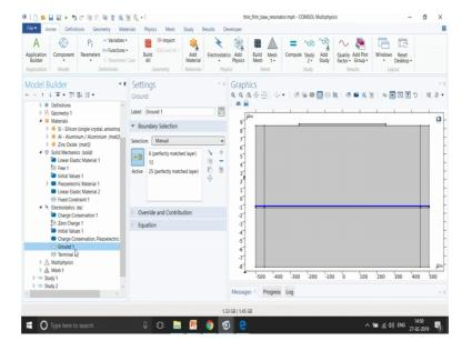
And, we have used a ground boundary condition on the bottom of the zinc oxide ok. And, then finally, we have used a multi physics node which actually couples the solid mechanics with the electrostatics ok. What I was telling you before is the use of PMLs.
