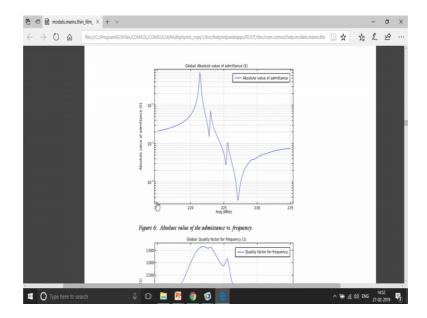
And, then this one talks about the admittance versus frequency. So, here we do a sweep of the frequencies from 215 to 235 and how does the admittance look with the sweep of the frequency.
