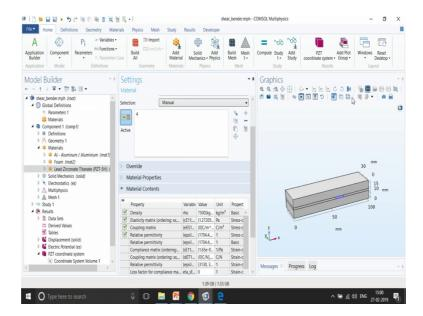
And, then finally, the PZT-5H and here we give a tensile material properties as you can see over here the blue part.
