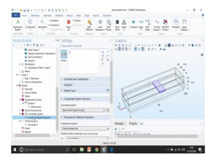
Finally, you can see that in this particular case we is very important example because in this piezoelectric we have used a different poling direction. So, by default you will see the poling direction of the any of the material properties is along z-direction.
