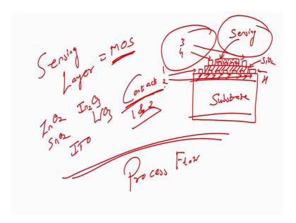
So, let me just show it to you, again if you can go back to the slide. So, what are we were talking about, we were talking about that we have a sensor, and sensor has four points. So, the first point should be a heater, first two points should be heater right. These are the contacts to the heater, heater contact 1 and 2 right. This is 1 and this is 2.
