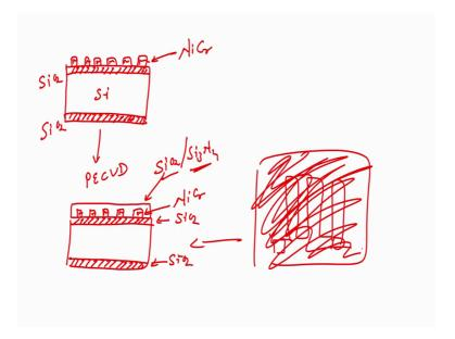
So, once I have a substrate with micro heater, let me draw it here all right. This is all silicon dioxide, this is silicon, silicon dioxide, silicon dioxide, this is our nichrome heater ok. Now, what we will do, we have to have insulator, because we cannot directly deposit metal oxide semiconductor on the micro heater.
