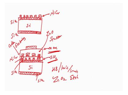
Only in this area because I used a bright field mask with a positive photoresist and that is why the unexposed region became stronger. After this I will go for hard bake 120, 1 minute, and then I will dip this wafer in zinc oxide etchant. I will dip this wafer in zinc oxide etchant.
