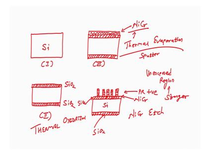
When I dip this wafer in nichrome etchant, what will happen? The area which is protected by photoresist area which is protected by photoresist will remain, and the area which is not protected by photoresist will get etched all right.
