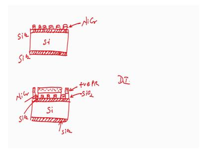
Now, I can access my heater right now I can access my heater. But, what I should do with this photoresist, I have to strip off the photoresist. So, after BHF after I rinse it, every step understand that you are there is a rinsing ok.
