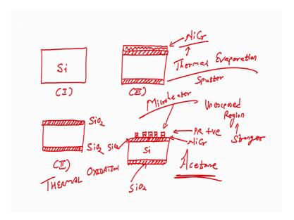
After nichrome etching, next step is I will dip this wafer in acetone, I will dip this wafer in acetone why, because when I dip this wafer in acetone, I will strip off my photoresist, I will strip of my photoresist. Now, what I have is a sensor or as a with a substrate with a micro heater, I have a substrate with micro heater. But, what I want? I want a substrate with micro heater this is your heater context 1 and 2 right, and a sensing layer and electrodes right.
