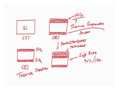
So, let us see the process flow. We start with a substrate start with a substrate which is silicon, then we grow oxide, so this is stage 1, stage 2. Stage 3, how you grow oxide, we grow oxide with the help of thermal oxidation all right, this is our stage 3. Stage 3 what we do? We will deposit a metal, this metal is for our heater, so I will say nichrome alright.
