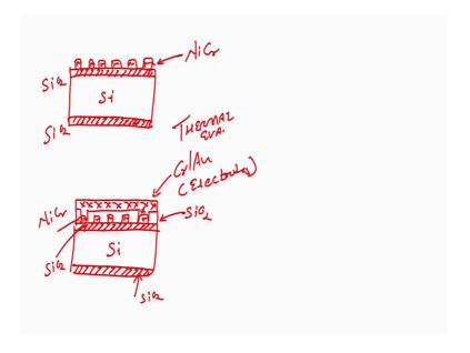
So, on this what I will do I will after this the next step would be I will deposit a metal. So, let me have pattern for metal as xx. This metal is for less this is chrome gold. This chrome gold is for electrodes. You can see right there are two heater context now I want to have electrodes. So, for electrodes, I will first deposit the metal using thermal evaporation, evaporation alright. After depositing metal the next step that I will perform is photolithography.
