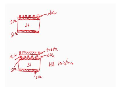
If I go for hard bake, the next step would be, I will dip the wafer in BHF. BHF stands for Buffer Hydrofluoric Acid. If I use BHF, what will happen, I will etch the silicon dioxide from the contact region from the contact region which is my heater contact, see there is no silicon dioxide you know there is no silicon dioxide in this particular area.
