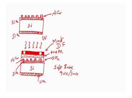
Now, let us see, how we can do that all right. So, after this, we will have photoresist. So, if I write it down, so you do not get confused, this is my insulating material, let us say silicon dioxide. This is my heater, which is nichrome, this is again silicon dioxide, which is thermally oxide, this is silicon dioxide, again thermal oxidation, this is my silicon, which is my substrate, and this is my positive photoresist right.
