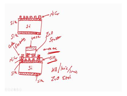
If I dip this wafer in zinc oxide ZnO ZnO etchant or ZnO2 Zno etchant, so, if I dip this wafer in zinc oxide etchant, what will happen I will have zinc oxide only on this area
