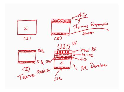
Next step is so you let me write down here, this is my photoresist right. This is my nichrome, this is silicon dioxide, this is silicon dioxide silicon and on this, I will have a mask. And that mask is my brightfield mask, you have seen in the lithography section right, what is the importance of brightfield, what is the importance of dark field right. So, this is my bright field mask, and this photoresist is positive photoresist ok.
