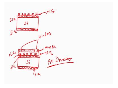
Next step is I will expose this wafer with UV light. After exposing, my next step would be, I have to develop the wafer for developing wafer we have to use photoresist developer right. So, if I dip this wafer in photoresist developer, after unloading the mask, and after UV exposure, what will I have? I will have my photoresist in the area which was not exposed by UV. And you can see here the windows for the contact to the micro heater are opened.
