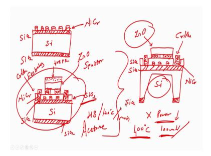
What does it mean if I etch the silicon substrate with bulk micromachining right, then now I have to heat sorry for the design like this all right, this is the kind of little bit better than earlier one ok. Now, I had to heat thin a thin layer of silicon and that is why I have my power to heat the semiconducting oxide will reduce. So, to obtain 100 degree centigrade or let us say 400 degree centigrade earlier was let us say 100 milli watt of power we required.
