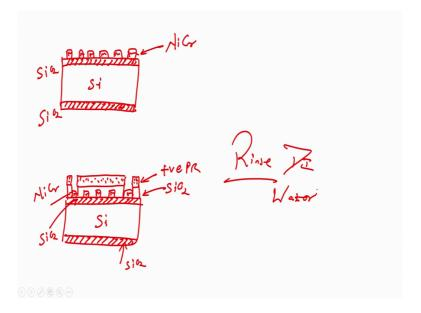
You have to washed wafer with DI water, you have to rinse the wafer rinse r i n s e wafer with DI water DI water. To every step, you have to go for rinsing with DI water.
