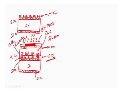
What is the next step, next step is I will deposit my sensing layer which is my metal oxide semiconductor, let us say Zn O sensing layer all right. How will I deposit my sensing layer, by sputtering? You take a zinc oxide target and then sputter it to form a film of zinc oxide, but do we require film oxides everywhere, no we only want film to be on this particular electrode, and the context should be open.
