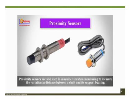
Proximity sensors are also used in machine vibration monitoring to measure the variation in distance between a shaft and its support bearing.
