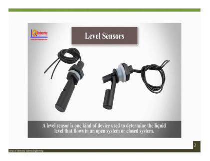
A level sensor is one kind of device used to determine the liquid level that flows in an open system or closed system.
