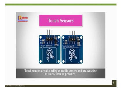
Touch sensors are also called as tactile sensors and our sensitive to touch force or pressure.
