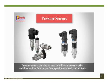
Pressure sensors can also be used to indirectly measure other variables such as fluid or gas flow speed, water level and altitude.
