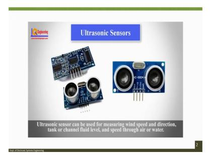
Ultrasonic sensor can be used for measuring wind speed and direction tank or channel fluid level and speed through air or water.
