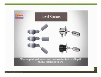
Whereas, point level sensors used to determine the level of liquid whether that is high or low.
