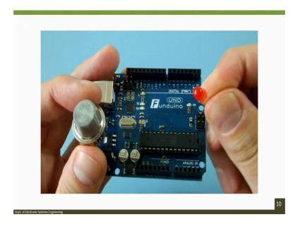
We will be reading values from the sensor and make the Arduino light an LED when gas concentration rises above certain level to build this project you will need a few things.
