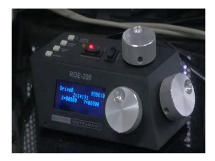
You can manipulate the movement using these are on the, the control system of the micromanipulator the z, x and y arms and you could also choose the 1 and 2 option, and then set the distance. So, this we have just tested for the third well, that are multiple devices, which are in the single chip here. All of these can be tested for the proof if you
