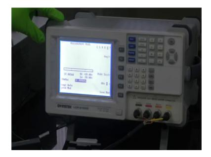
So, this is the LCR meter or the impedance analyzer as you can see like I mentioned this is a four probe device.
