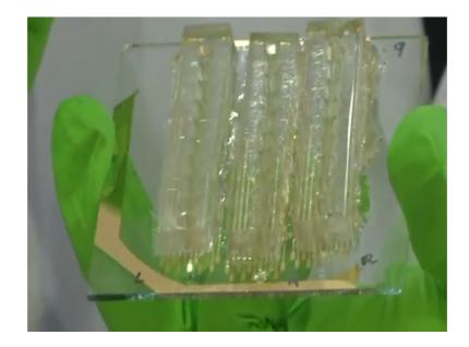
So, here this one example of a sensor; so, this is the biosensor so this is the biosensor in my hand, which measures the impedance. So, we call it an impedance biosensor and this is used to test the antibiotic susceptibility. So, what happens is how do you do the impedance test like, you could see here there are electrode pads.
