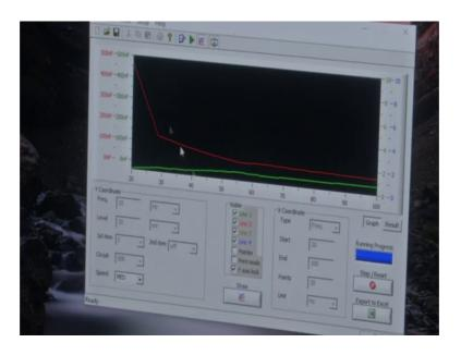
Let us do the frequency sweep and check the impedance measurement. As you see there is the drastic change in the measurement here. So, this was the empty well and here. So, as you can see this is a capacitance here. So, we have change the item which is measuring here is the capacitance. So, we need the impedance measurement.
