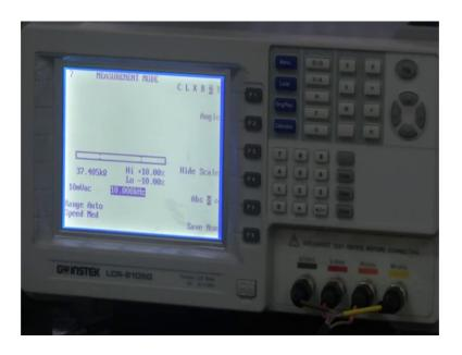
We can select they are different frequency range, you could chose all frequency. And now the two leaves the two electrodes in my hand, I will open circuit configuration and then we do the OC trim. Now, that this complete let us do the short circuit trim.
