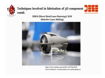
DMLs utilizes a variety of metal and alloy materials such as stainless steel cobalt chrome and inconel to create strong durable parts and prototypes. DMLs is an excellent choice for functional metal prototypes high temperature applications and end use parts.
