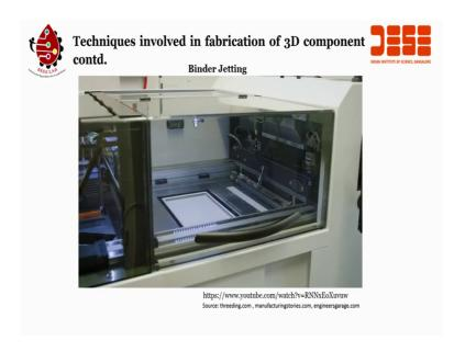
In this process, a liquid binder is selectively deposited on a powder bed with a print head. It is a growing process that allows the production of parts for the manufacturing medical and dental industries. This technique enables the production of metallic and ceramic parts as well as sandal stochastics. Just try the process a 3D drawing is imported into the printer software.
