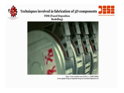
It is a fancy word for laying down a small bead of plastic what is really cool is you can have a real engineering grade thermal plastic. So, the same stuff you would injection mold. Someone needs a ABS or polycarbonate or a high temperature ultem. We can actually print it directly as opposed To casting a partner into having a ejected molded parts done.
