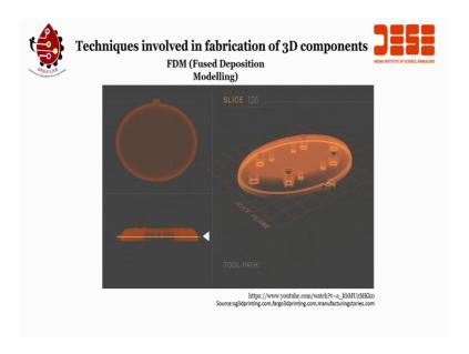
The raw material is produced into a filament like fishing line type one that filament is wrapped around a spool. So, that is your cartridge of raw material that is going to be used to build parts. That material then gets fed up through the machine all the way to the head where it is liquefied and extruded in fine layers. The support material is extruded at the
