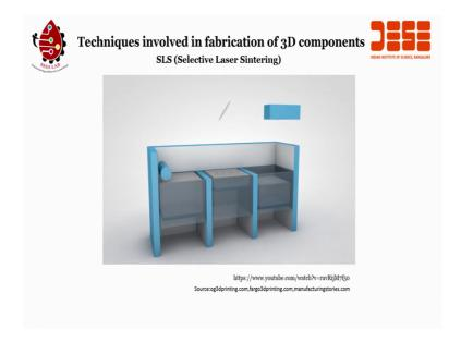
Once the nylon powder is loaded in the supply container and digital instructions, are programmed the laser unit directs a high powered beam to a reflective mirror. From there the galvo motor system steers the focused beam to the powder surface, each layer of part geometry is then sintered into a heated bed of nylon. Pistons move the supply container up and the build chamber down while the roller moves across the bed to distribute the next layer of powder.
