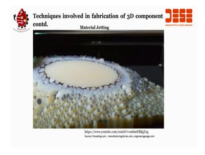
And so layer by layer complex models takes shape. The most advanced PolyJet systems can built multi material parts soft, rigid, clear and colorful.
