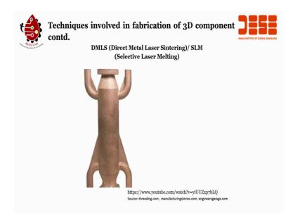
The DMLs process begins in the same fashion as other layer additive manufacturing technologies. A program takes 3D cad data and mathematically slices it into 3D cross sections each of these sections will act as a blueprint telling the DMLs machine exactly where to center the metal material. The data is then transferred to the DMLs equipment.
