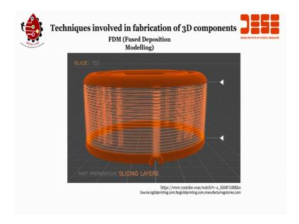
Our software it takes a 3D data file and it slices it into the layers, then creates a tool path that is sent to the machine.
