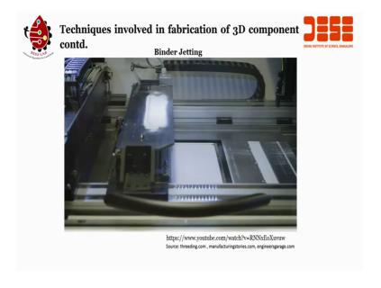
First a powder layer of a specific thickness is prime. Thereafter the printing head moving on two axes projects the binder wears necessary. Before moving on to the next layer the solvent contained in the binder is evaporated by an Indian their supplier. The powder bed is then lowered and a new powder layer is deposited. Therefore, the production takes place in a series of steps that build the part layer by layer. When the cycle is completed
