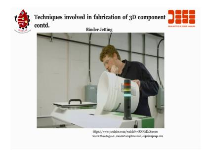
The powder to be used is placed in a dispenser which ensures a constant supply during printing.
