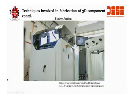
Binder jetting additive manufacturing is a process inspired by the technology of inkjet printers.
