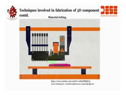
They works like an ink jet printer, but instead of jetting drops and ink PloyJet pretty printed is jet tiny drop us liquid plastic. A UV light is an liquid plastic solidifying it.
