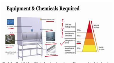
Bio Safety Hood/Cabinet: This is where the primary tissues will be processed to obtain the cell culture. It is equipped with all precautionary features to eliminate contamination as well as hazard to the personnel handling the tissue. The different essential parts of a biosafety hood are shown. There are different biosafety levels depending on the type of organism that one works with. This is tabulated above.
