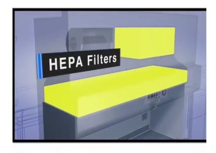
It includes HEPA filters for exhaust and supply air.
