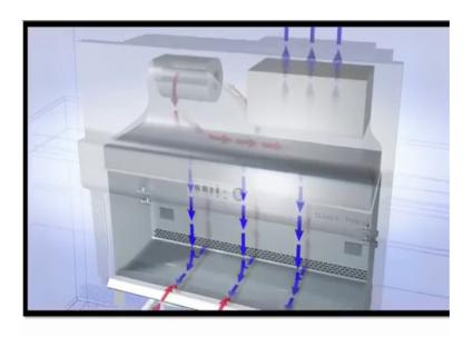
Then through the HEPA filters 30 percentage of the filtered air is exhausted, the remaining 70 percentage which is now HEPA filtered is recycled back into the workspace to ensure maximum protection.
