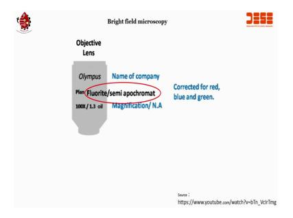
The term fluoride or semi apochromat means the lens is corrected for three colors; red, blue and green.
