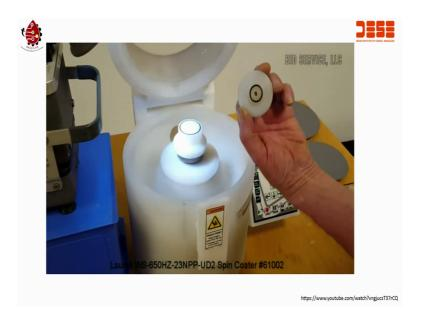
Next, we are going to spin a small wafer. It has this very-very nice little adapter here, that you can fit right on top with the standard chuck raspberry pi vacuum.
