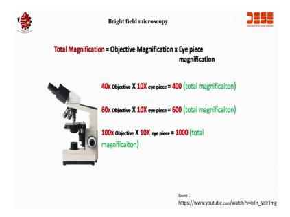
The total magnification of the specimen observed as the product of magnification of the objective and the magnification of the eye piece.
