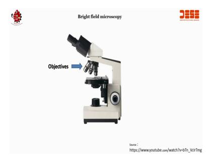
Now, let us talk about objectives. The objectives are the most important imaging components of the optical microscope and play a key role in magnification and resolution of the specimen. All the objectives have an information written on it.
