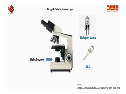
The light source can either be a halogen lamp or an LED.
