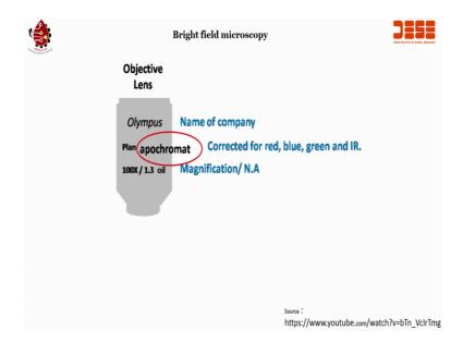
And the term apochromat means the lens is corrected for four colors; red, blue, green and infra-red.
