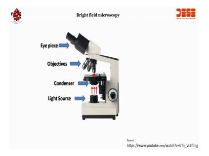
The condenser collects the light from the light source and directs the light to specimen, which is kept on the stage. The light passing to the specimen is collected by the objective lens and the final magnification is created by the eye piece.
