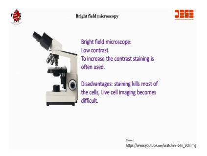
Bright field microscope typically has low contrast, as most of the biological samples transmit most of the light. To increase the contrast staining is often required. The disadvantage of staining is that most of the cells are killed and live cell imaging is difficult. Now, since here used the right field and seen the bright field microscopy, let us also see the fluorescent microscopy and let me play the fluorescent microscopy as well.
