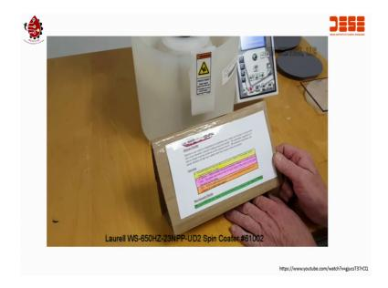
I have this chart here and this is wafer size versus spin speed um; obviously, the smaller the workpiece the (Refer Time: 42:59) need to spin and I given a little guideline here, first we ran (Refer Time: 43:04) up to 12000. Now, we are going to run a 100 millimeter wafer as suggested up to 6000.
