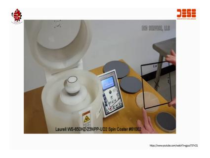
However, what is important also in particular unit, is that has the capability of spinning a 4 5 inch by 5 inch square substrate. I have a piece of glass here.
