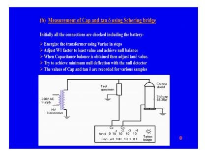
This is again a second type of bridge for like a transformer ratio arm bridge, which is known as a Schering bridge; here transformer high voltage transformer, again the test specimen which is to be measured the capacitance; is to be measured and again is connected here. The Cn being the standard capacitor in here, in present case; the standard capacitor being 68.35 picofarad with a hydrogen filled insulating media.
