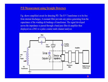
So, how the circuit looks partial discharge measurement, there are different partial discharge detectors which are being employed by the utilities or the laboratories where the equipment is being tested or the partial discharge measurements are being carried out. So, for partial discharge measurement you should have a laboratory without any interference and the circuit details are shown here for the measurement.
