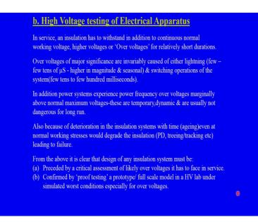
So, that was about the non-destructive type of measurements which are to be carried out for the insulation. We look into the high voltage testing of various apparatus, this is essential as in service an insulation has to withstand in addition to continuous normal voltages, sometimes higher voltages or over voltages for a short durations.
