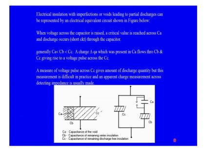
So, these measurements have to be carried out at regular intervals and to check the healthiness of the equipment which is in service. How partial discharges or estimated or calculated, so in electrical insulation with any imperfections; which is not properly done or has containing a voids, this could lead to partial discharges this is; in case of a insulating material could be represented by an equivalent circuit simple equivalent circuit as shown in the figure a below here.
