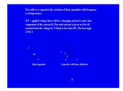
So, for a capacitor or a cable; the variation of the quantities, the applied frequency and the voltage is of importance. So, if in case considering a viewing the applied voltage there will be a charging current; consider here the charging current which is shown here I s, I c charging current for I c and a loss component of the current; the loss component of the current is Il; Il is shown here; Il is a loss component.
