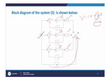
3 integrators integrator 1 integrator 2 and 3 y 3 integrator because you have 3 states x 1 dot x 2 dot and x 3 dot these summation blocks now this is the input. This c 1 c 2 c 3 which we have determined here c 1 c 2 c 3 and here specifically see b 3 into u
