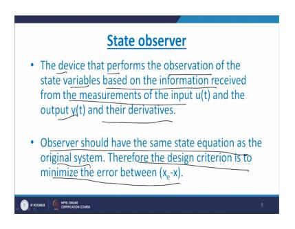
The observation of the state variables base on the information received from the measurement of input and output and their derivatives then second point observer should have the same state equation as the original system therefore, design criteria is to minimize the error between X e and x. So, we already seen that here see here that we require the error between X and X e should be minimum.
