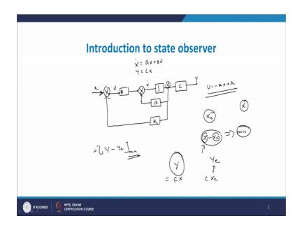
Let us say X dot equal to A x plus B u this is your system; now here say an integrator, now here is our C matrix and here is output y here is X dot, now here is B and input U and here is matrix A. So, here X dot equal to A x plus B u and y equal to CX. Now, when we talking about the controller design, so controller design basically is state space is with respect to state, now here this is a state x here.
