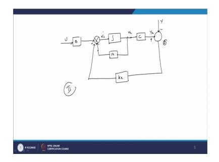
Now, will draw the block diagram of this state observer, now here is estimated state X e dot and now here is X e; now here B input U here is A matrix, now here is C matrix and as state X e is the estimated state therefore, here output is instead of Y it is Y e and here Y e is the output. And next the output Y which is coming from the actual system you just see here. Here this output is coming here this output is coming and it is shown here this output Y e is the estimated output.
