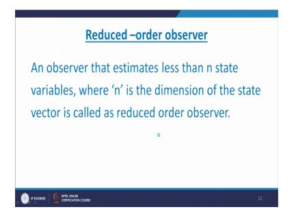
And similarly the reduced order observer reduced observer means there are some states which are known which are unknown. So, what we are doing the states which are which can be possible to measure we are measuring it and which are only unknown that only estimating that is called reduced order observer.
