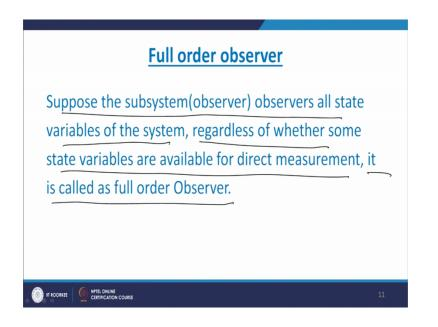
So, suppose the subsystem observes all state variable of the system regardless of whether some state variables are available for direct measurement it is called as full order observer. (Refer Slide Time: 25:33)
