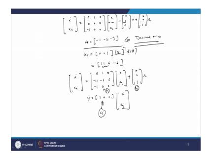
We have to write the elements of A elements of C x x a B 0 and we see the equations as the model is x dot x a dot 0 1 0 0 0 0 minus 1 0 0 here is x x a 0 1 0 u and here 0 0 0 1 into r. This is the state space model of the system when there is we can say no controller and we have got this results x a plot is the part of the integral controller, now our purpose is to design a controller suppose our pole plus pen we are debian or minus 1 minus 2 minus 3. So, this indicate your desired poles.
