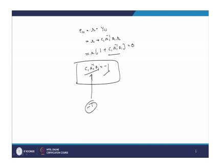
Now, about the steady state error; Steady state error e s s is given as r minus y s s. So, here we can write only this as r plus C 1, A 1 inverse, B 1 into r and here you take r is common you get 1 plus C 1 A 1 inverse B 1, B B 1 equal to 0. So, here steady state error is to be 0. So, when this is possible. So, this is possible when this is the conditions C 1 A 1 and this B B 1 equal to minus 1. So, this is the conditions.
