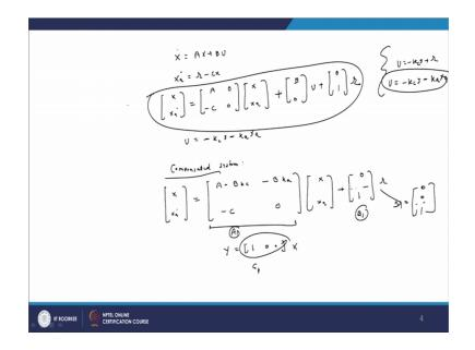
Now, we see now will see state equation as X dot equal to Ax plus Bu; this is the state equation for the original plant and because the new state has come. So, here the equation is x a dot equal to r minus c x you will find at here x a dot equal to r minus y that is here this x a dot equal to r minus here y here r y c into x. Therefore, here you got x and x a dot and if you combine this equation x dot x a dot here A 0 minus C 0 that is x here is x a plus B 0 into u plus 0 1 into r.
