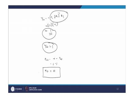
So, particularly C 1 A 1 inverse. So, if you use the values of A 1 B 1 and C 1 we have find that will get here minus and you get this minus 1 here will get minus 1 it is (Refer Time:26:58) as 1. So, steady state error or steady state output we comes to be 1; that means, you are the error the steady state error e ss equal to r minus Y ss that is 1 minus 1 that is steady state error equal to 0.
