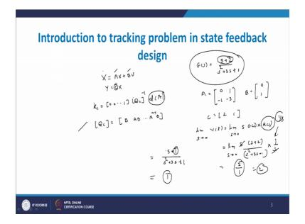
Now, we have seen state feedback control design. And we have seen that for state feedback design there is for X dot equal to AX plus BU Y equal to say C X, the controller k controller k c is determined as 0 0 0 1, a controllability inverse phi of A. And here this controllability matrix Q C is repaired by B AB A raise to n minus 1 b. So, we will find that the controller in a state feedback design is depends upon B matrix, A matrix, and phi of A is the desired characteristic equations.
