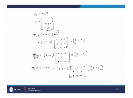
So, now they need to determine the transformation matrix T. So, here K c equal to K c m into T we can write down as this T equal to T 1 T 1 a T 1 a square. So, this T 1 equal to 0 0 1 Qc inverse controllability inverse and we have already determined the controllability inverse like this and 0 0 1 is there. So, if you multiply this 0 0 1 and Qc inverse which we already determined we can write down as minus 1 2 1 1 1 0 1 0 0 if you solve it will get 1 0 0.
