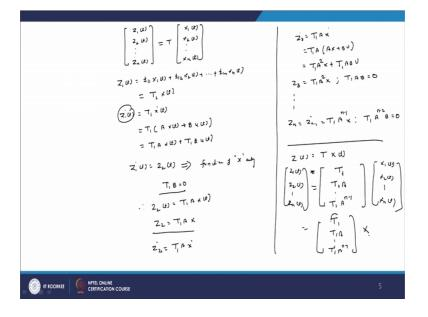
So, now here the states is there that is represented by Z 1 t Z 2 t Z n t; n states. Now here this is a transformation T and state say in terms of time T x 1 t x 2 t say x n t. So, now here there are n states that is z 1 z 2 z n and x state x 1 x 2 x n, these are the original states these are modify states.
