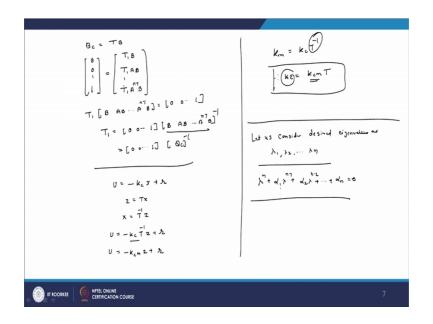
So, here we can write down as this B c equal to T into B. So, this B c is 0 0 say 1 and conditions of T is say T 1 B T 1 into a B and here T 1 A raise to n minus 1 into B. Now if you solve it so, you will get T 1 B A B A raise to n minus 1 B equal to 0 0 0 1 and hence this T 1 equal to 0 0 1 as B A B.
