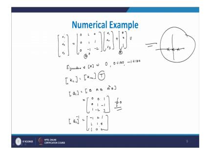
Now, we start solving some numerical example base on this technique. So, now, our example is x 1 dot x 2 dot x 3 dot equal to  $0\ 1\ 0\ 0\ 1\ 1\ 0$  minus 1 minus 2 x 1 x 2 x 3 plus 0 0 1 into U. Now the Eigen values of this matrix A, this is matrix A, this is matrix B. The Eigen values of this matrix say r Eigen values of a belong to 0 0 point 6 1 8 0 minus 1 point 6 1 8 0. We know that Eigen value govern the performance of the system.
