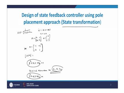
Now design of state feedback controller using a pole placement approach that is state transformation. Last time we have solved system or we have solved one example, in an example we have seen that the our given system that is x dot is equal to A X plus B U Y equal to c x.
