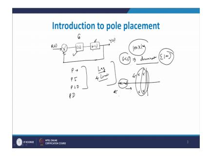
Introduction 2 pole placement basically what is mean your pole placement pole placement means that we have design a controller. It is similar to the controller which we are design in a classical approach. For example, in classical approach what we are seen? We have a plant it is like this.
