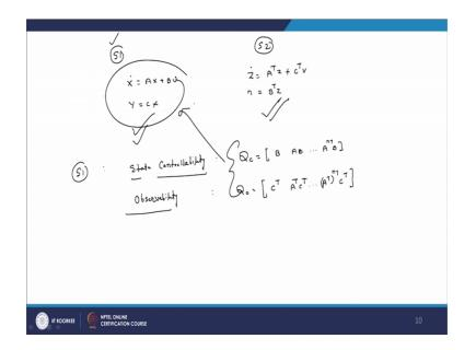
So, this way I have written s 1 here; for s 1 i have we have to take a one model suppose this model is represented by x dot equal to A x plus B u and y equal to C x this is system s 1 this s A is system matrix B is input C is the output matrix.
