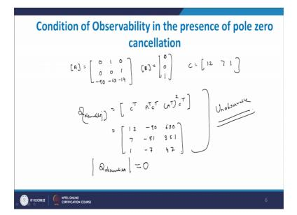
Suppose if you write A matrix as this A is equal to 0 1 0, 0 0 1 and here minus 90 minus 63, minus 14, this is A matrix now here we write a B matrix as 0 0 1 and C matrix as 12 7 1. So, steps involve A B C. So, we have to an a b and c now we have to check the
