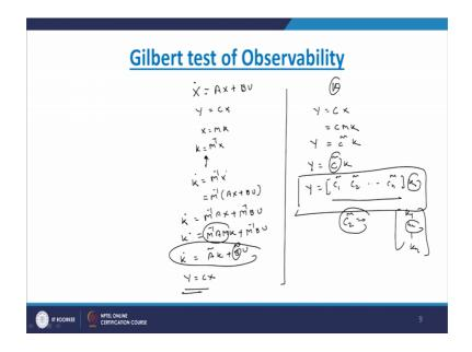
So now, this concept is base on diagonalizations. So, I am taking a model as X dot equal to A X plus B U and Y equal to C X. So, X dot equals to ax plus B U Y equals to C X and now the concept of diagonalization is based on state transformation. You can take any other state, you can assume any variable. So, for as we are assuming the variable K every times earlier also here also we are assumed with assuming a new state in terms of k. So, here you can take X equals to M K.
