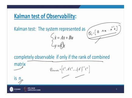
Now the next thing mathematically how to check the observability of the system? And observably is there an observability means this concern with the output. Therefore the important role of C is here. We have seen that in case of state controllability, the control state controllability Q C, there is a involvement of only B A B A raised to n minus 1 B.
