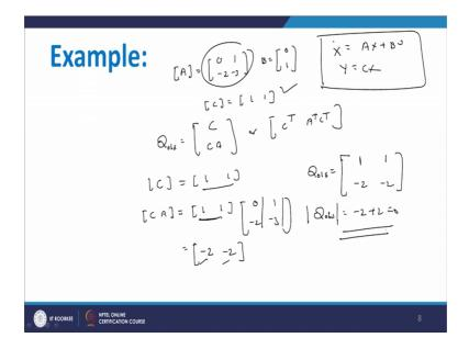
Now we see example. So, we have taken simple system. So, let us say A matrix as 0 1 minus 2 minus 3 and say B matrix as 0 1 and our C matrix is like this C equal to 1 1 and this plant is nothing, but X dot equal to A X plus B U and Y equal to C X. Now our main purpose is to check the observability of the system. We are check controllability as well as up to controllability of such type of example.
