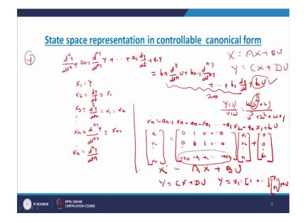
Now, we have to represent the given system in a state space form. So, state space form is, we want to system to be in this form X dot equals to A X plus B U, Y equals to C X plus D U, this we want.
