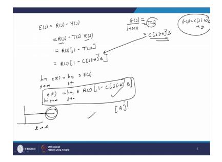
This E of s equal to reference input that is R of s minus Y of s and Y of s we have already calculate. So, just shifting this Y of s here or placing this Y of s here we will get R of s minus T of s into R of s.
