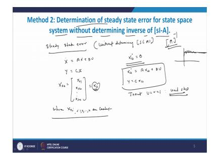
So, we can see this method. So, method two, determination of steady state error for state space system with the how determining in the inverse of sI minus A. Now, here this method is explaining. So, we will find that here also we need to get the inverse, but it is not sI minus A here in this method only there is need to get the inverse that is A inverse only, this part sI, sI part we can remove.
