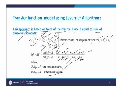
Now, this approach is based on trace of the matrix, trace is equal to sum of diagonal elements so here a 11 a 12 a 1 3 first row, a 21 a 22 a 2 3 second row, a 31 a 32 a 33 this is a third row. So this is a given matrix this is matrix A.
