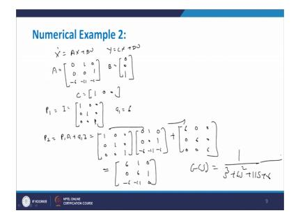
So, here if you write A as  $0\ 1\ 0\ 0\ 1$  minus 6 minus 11 minus 6 B equal to  $0\ 0\ 1$  and we have C that is equal to  $1\ 0\ 0$  A B C we have written. Now what is our first step first step to get P 1 and then a 2 and like this the first part is to get the P 1, so we write P 1 equal to I that is a identity matrix that is equal to  $1\ 0\ 0$ ,  $0\ 1\ 0$ ,  $0\ 1$ .
