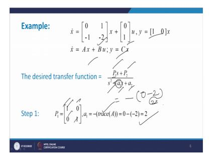
So, x dot equal to A x plus B u and what is the desired transfer function? My desired transfer function is P 1 s P 2 s square a 1 s plus a 2 this is required to be determined. Now to how to get a P 1 how to get P 2 how to get a 1 and how to get a 2 now P 1 you just see the first step P 1 equals to I that is a identity matrix.
