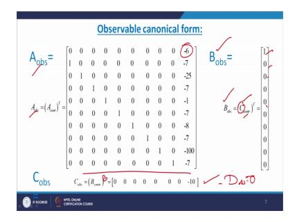
Now, about the observable canonical form; last time I have explained. Observable canonical form is also useful in state space analysis particularly in checking in checking observatory, also when we need to design observer, this type of form is useful. Therefore, here we have written the observable canonical form for this particular system; but will be write the observe form, it is better. First of all, we write in a companion form and then you convert it because it is very easy.
