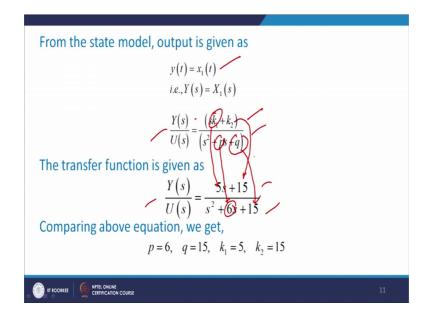
So, here that is why we have written here Y of s equal to X 1 of s and this is Y s by us like this and now we have compare. So, after comparison will find at this is p; p s this is 6 s. So, p corresponds to 6; Now, here q; this q corresponding to 15 and this k 1 corresponding to 5 and k 2 corresponding to 15. So, in this way, we have determined the unknown in the state space model. Now we start with the, another example.
