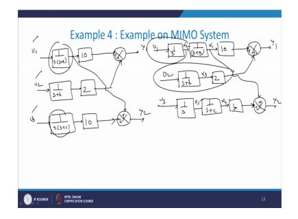
Now, here we solve an example where here we show that for a MIMO system also, we are getting this state model in a first order form. So, we start doing this example, see now here I am taking one block U 1. This is one input; 1 upon s s plus a. Now here I using 10; then here is a block I am showing. Here is Y 1. Now, another input is coming that is U 2 and here that transfer function is s plus b. Then here, is 2. Now it is connected here.
