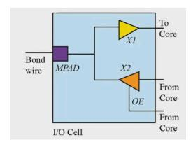
So in this figure I am showing you a bi-directional IO cell. So in an IO cell there is a metal MPAD which I am showing this is a metal through which a connection is made. So from this metal the wire will go to the package that will show in the next slide but understand that this is the IO cell and inside this IO cell there will be some metallic pad through metallic contact from this the wire will go to say one buffer and another buffer.
