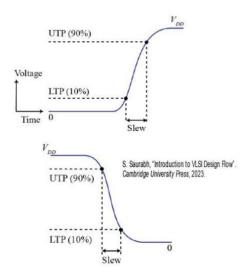
So based on this definition or this choice of our threshold point or transition point how do we define slew? So we define that the slew can be for different for the rising and the falling case. So in this case, since the signal is rising, we say that this is a slew and this is
